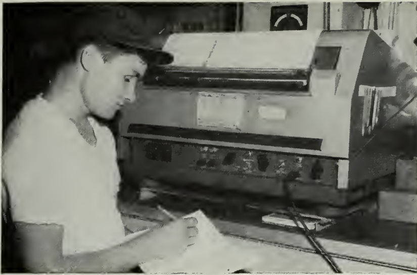
DEPTH Recorder automatically measures ocean's depth with electronic beam.
